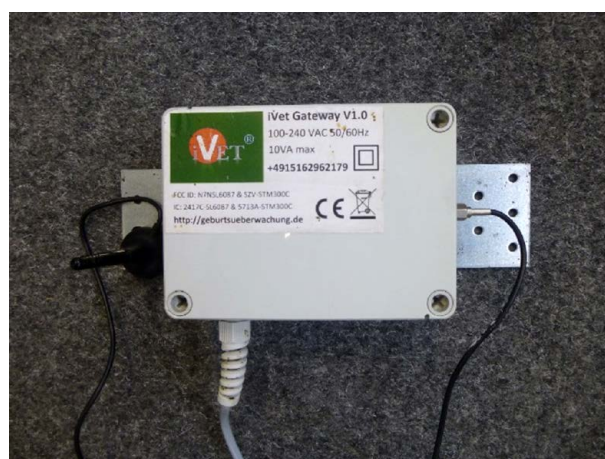
Fig. 2. Receiver unit of the iVET ® birth monitoring system
