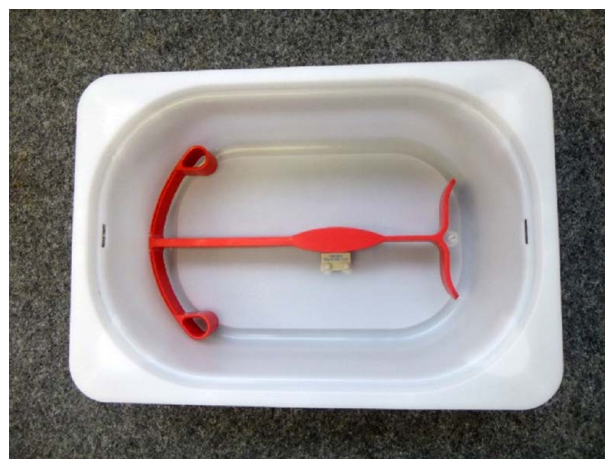
Fig. 1. Transmitter of the iVET ® birth monitoring system
